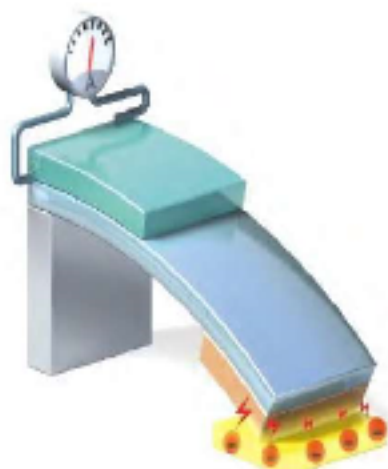
Fig 3. When the cantilever bends to the point where the copper sheet touches the radioactive source, the electrons flow back to it, and the attractive force ceases
