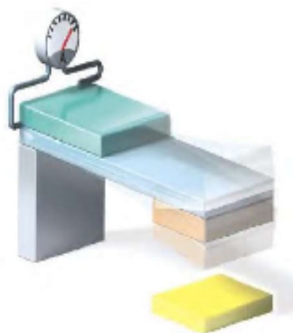
Fig 4. The cantilever then oscillates, and the mechanical stress in the piezoelectric plate creates an imbalance in its charge distribution, resulting in an electric current
